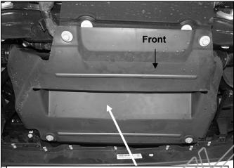
(Fig 1) Remove splash guard or skid plate from
