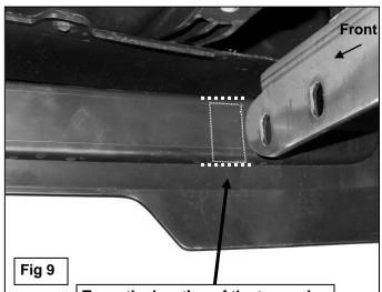
Trace the location of the top and bottom of the Frame Bracket onto back of spoiler and cut out to clear mounting tabs on Bull Bar
