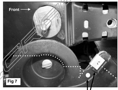
Move metal clip to here (See Dot) after cutting OR drill a 1/4" hole and replace the clip with the included:
