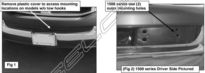
Example of Ram 25-3500 (and 1500 Mega Cab) Series Driver Side Installation Pictured
