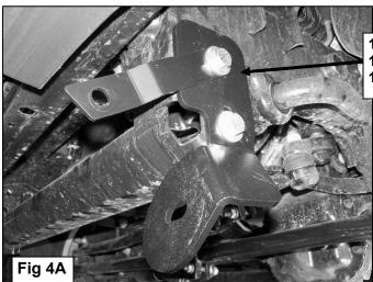
12mm x 40mm Hex Bolt 12mm Lock Washer 12mm Flat Washer
