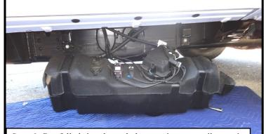
**Step 6.** Carefully bring the tank down trying not to tilt or twist the tank to avoid damage to connectors.
