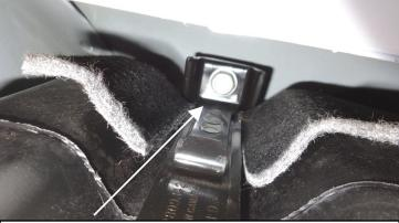
**Step 4.** Using a ratchet with a long extension and a 13mm socket loosen and remove the bolts of the tank support straps. (depending on model, bolts may be 13mm head socket or Torx T-40 bit.)
