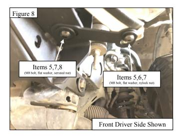
10. Install the skid plate for the Pro-Series Bumper using the provided M8 hardware (5,7-8). See Figure 9. 10, and 11 for reference
