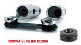
Interchangeable pushrods seats (offsets available) enable customized oil flow, while the EDM oiling hole feeds oil directly to the needle bearings.
