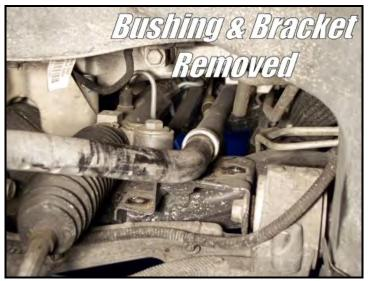
Turn the steering wheel all the way to the left and fish the stock sway bar out the driver side.
