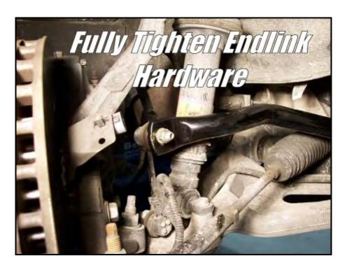
You are now finished with the front sway bar installation! Make sure that all hardware is fully tightened before driving the vehicle. Let's move on to the rear sway bar installation.
