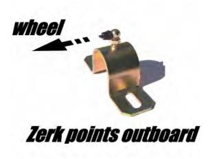
Insert the adapter block as shown in the picture. Install the provided longer bolt and washer. Reuse the stock bolt for the forward bracket hole. Fully tighten bolts.
