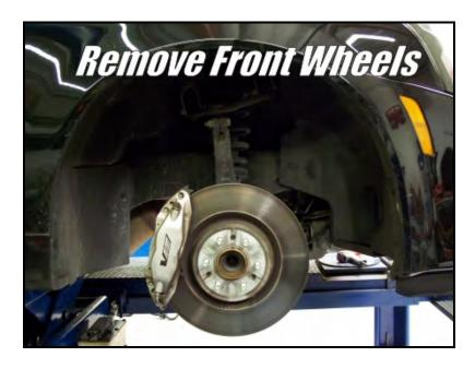
» Undo the sway bar end link nut using a 15mm socket. Retain this hardware for later use.
