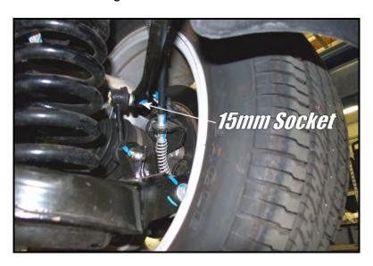
Undo the 2 subframe mount bolts on each side. Retain this hardware for later use.
