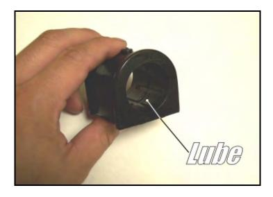
» Slip the bushings over the sway bar in the proper position. Slide the Hotchkis bracket over top the bushing. Install the stock hardware to secure the new bracket to the subframe. Fully tighten all hardware.
