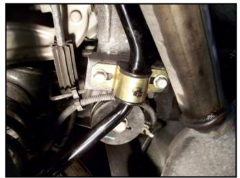
» Reattach the end links to the sway bar ends using the stock hardware. Fully tighten end link nuts.
