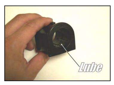
Slip the bushings over the sway bar in the proper position. Slide the Hotchkis bracket over top the bushing. Make sure the Zerk fitting is pointing towards the outside of vehicle.
