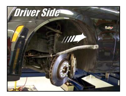
» Place the stock sway bar on the floor and set your new Hotchkis sway bar next to it. This will allow you to properly orient and position the bar for reinstallation.
