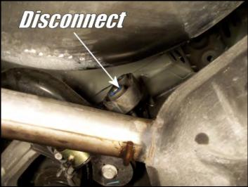
Remove the center brace located in the center of the car to allow the exhaust to drop even further.
