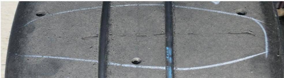
When it first appears, a visible tread splice is cosmetic in nature and does not negatively impact the safety or performance of the tire. The appearance of a visible tread splice is not a defect in the tire. However, unless appropriate steps are taken, this condition may result in an open tread splice, which will require the tire to be immediately removed from service and replaced.<sup>2</sup>
