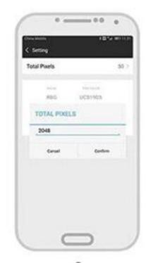
If pattern on Device is not even adjust Pixel # to total # of LEDs.
