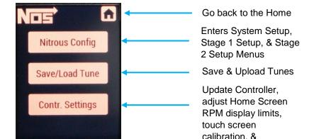
In the Nitrous Configuration menu, you will be presented with a choice of three menus – System Setup, Stage 1, & Stage 2. NOTE: The controller will come pre-programmed with default values. These are only placeholders and will need to be configured.
