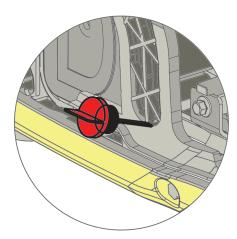
Insert a funnel into the crankcase dipstick hole and carefully add the specified amount of 4-Cycle engine oil (SAE 10W-30) to empty reservoir until or oil reaches the outer edge of the oil fill hole
