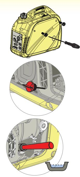
Do not tilt generator when adding oil. This could result in overfilling which could damage the engine. Make sure no foreign matter enters the crankcase.
