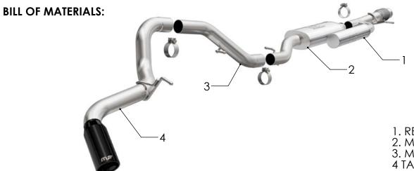
1. RESON ASSY 2. MUFFLER ASSY 3. MID PIPE ASSY 4 TAIL PIPE ASSY
