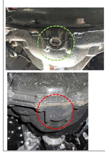
If the Differential has the drain plug the RS62116 will fit on your application.
