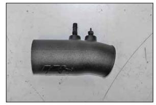
8. Install the provided NPT vent fittings into the K&N $^{\circ}$  intake tube as shown.
