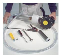
**Step 3:** Tighten snugly with the open end 9/16 wrench.
