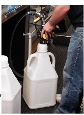
The next two illustrations display the squeeze clamp assembly being used. Before a fluid transfer operation, it is imperative that you apply the squeeze clamp to the object you are transferring fluid out of or into. It ensures that the hose will stay in the fluid opening.
