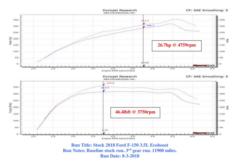
Run Title: K&N 2018 Ford F150 3.5L Ecoboost Run Notes: K&N boost module #21-2599 installed. 3<sup>rd</sup> gear run. 11900 miles. Run Date: 8-3-2018
