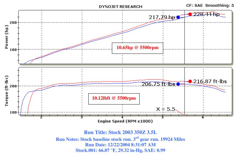
Run Title: K&N Intake Kit 2003 350Z 3.5L Run Notes: K&N Intake Kit #57-6013 installed. 3<sup>rd</sup> gear run. 19924 Miles. Run Date: 12/22/2004 9:35:51 AM K&N.002: 72.92 °F, 29.29 in-Hg, SAE: 1.00
