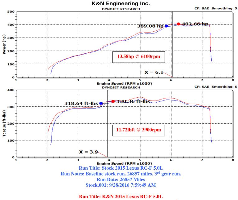
Run Title: K&N 2015 Lexus RC-F 5.0L Run Notes: K&N intake kit #63-9038 installed. 26857 miles. 3<sup>rd</sup> gear run. Run Date: 9/28/2016 9:09:47 AM K&N.002: 90.69 °F 28.97 in-Hg Humidity: 23 % SAE: 1.04
