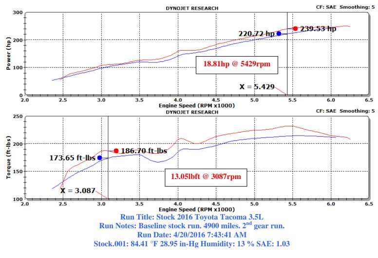
Run Title: K&N 2016 Toyota Tacoma 3.5L Run Notes: K&N intake kit #77-9039 installed. 4900 miles. 2<sup>nd</sup> gear run. Run Date: 4/20/2016 12:36:47 PM K&N.002: 97.25 °F 29.00 in-Hg Humidity: 6 % SAE: 1.04
