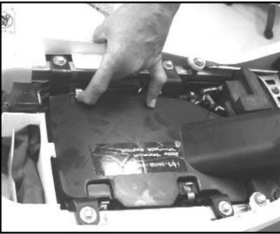
3. Unclip the four air box lid hooks.
