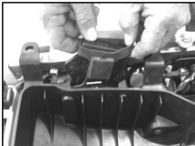
10. Remove the Engine Control Unit Assembly band.
