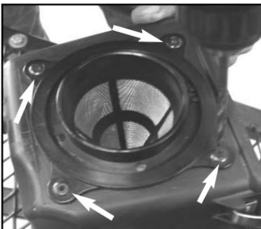
13. Drill out the four blind rivets from the air filter holder. **Note:** Do not use a drill bit larger than 7/32". Be careful so you do not elongate the air box holes.
