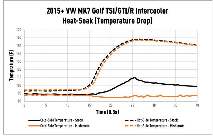
FIGURE 9: Temperature drop comparison during heat-soak test.
