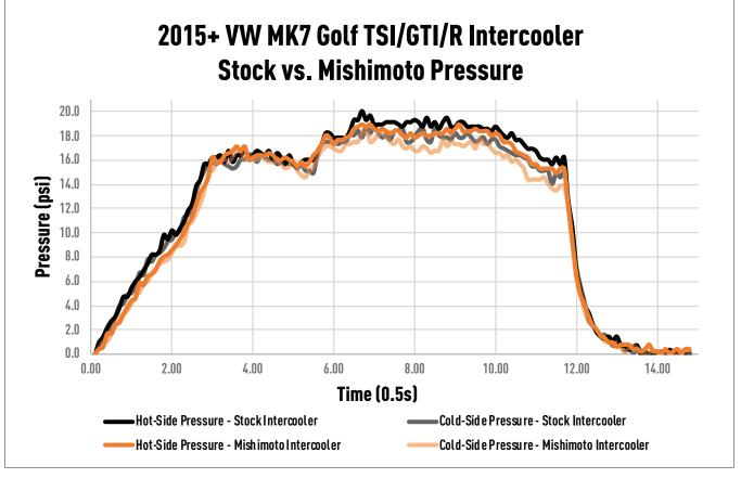
FIGURE 6: Pressure drop comparison.
