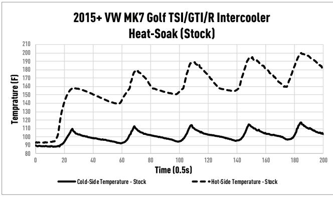
FIGURE 7: Heat-soak test.
