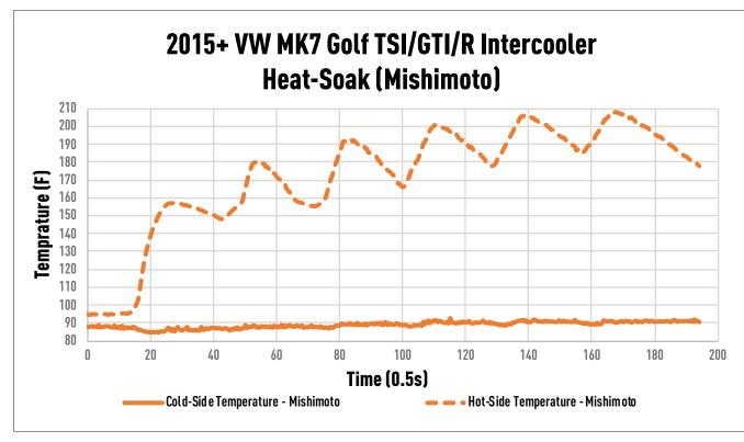
FIGURE 8: Heat-soak test.
