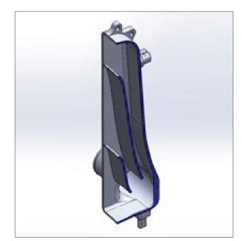
FIGURE 3: Two internal air diverters are integrated into the hot-side end tank.
