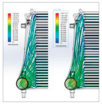
FIGURE 4: CFD comparison results, before and after the air diverters are added into the design.
