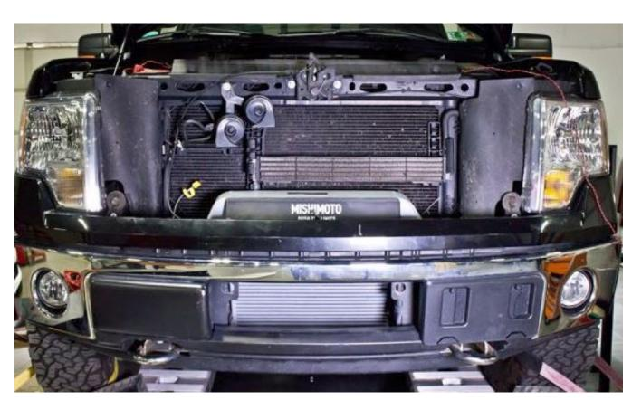
FIGURE 1: The Mishimoto intercooler features shrouding to direct ambient airflow through the core for maximum temperature reduction.
