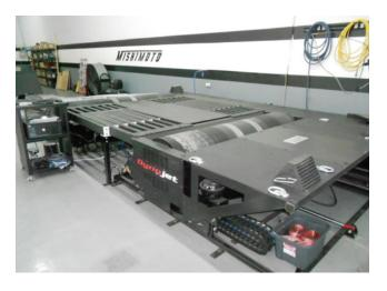
FIGURE 2: A Dynojet<sup>TM</sup> dynamometer was used for vehicle testing.
