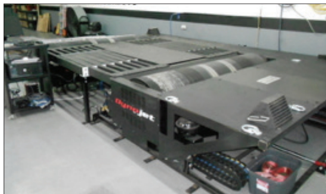
FIGURE 3: A Dynojet™ dynamometer was used for vehicle testing.
