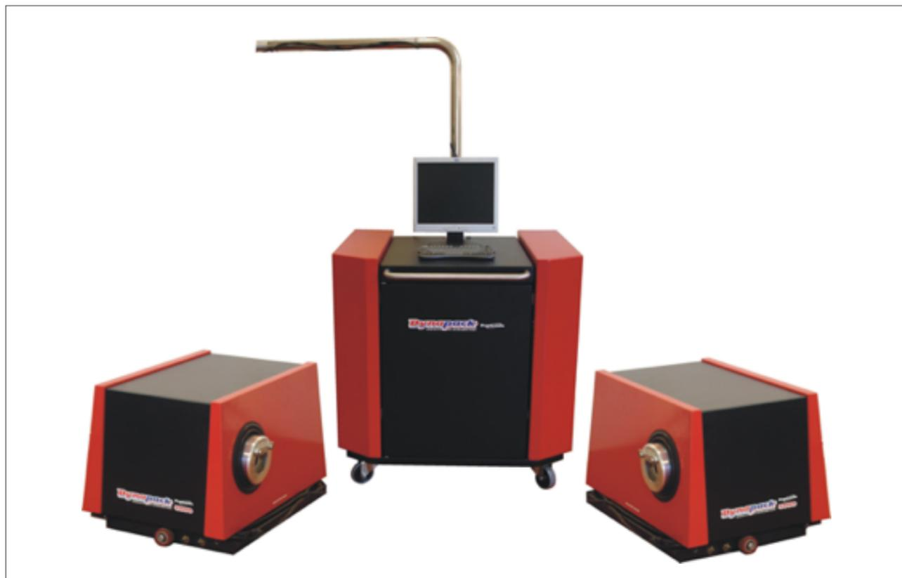
FIGURE 3: A DynaPack™ dynamometer was used for vehicle testing.
