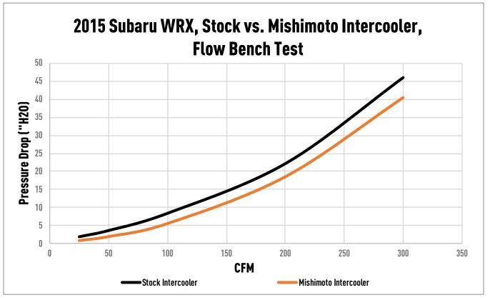
FIGURE 7: Flow bench test. At 200 CFM the stock core has a pressure drop of 22 H2O while the Mishimoto has a lower pressure drop of 18.5 H2O. The Mishimoto core is lower across the entire range of testing.
