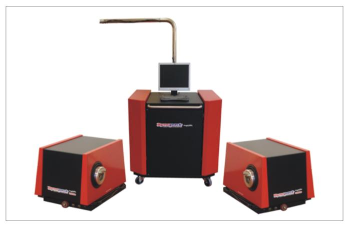
**FIGURE 3:** A Dynapack<sup>TM</sup> dynamometer was used for vehicle testing.
