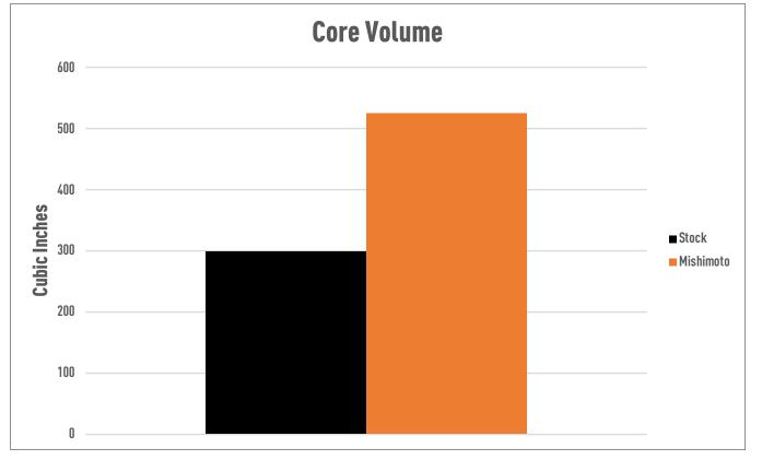
FIGURE 1: The Mishimoto intercooler core is 75% larger than stock while maintaining a factory fit.
