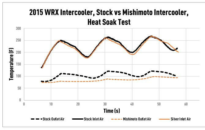
FIGURE 5: Mishimoto Intercooler Heat-Soak Test, notice how the stock intercooler temperatures are higher and rise faster than the Mishimoto core.
