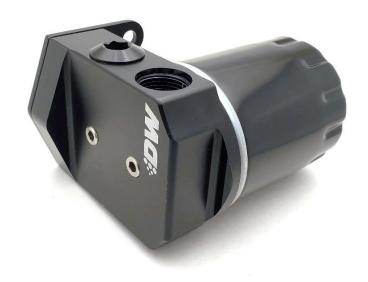
DW Spin On filters are compatible with pump gas, race gas, and ethanol. DW recommends a maximum service interval of 12 months or 12,000 miles. Shorter service intervals are recommended with harsher conditions and corrosive fuels. The DW SOF features dual -10AN O-Ring ports for plumbing flexability.
