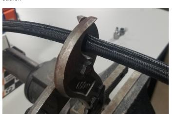
**2** During the cut you may crimp the hose. Make sure it's nice and round so the installing the nut that will go over it will be smooth.
