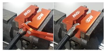
**6** Slide the nut up to the fitting and thread as much as possible by hand to ensure they do not cross-thread.
