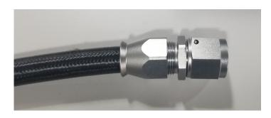
8 Make sure the nut is well secured and tight. Lining up the hex on the nut and the hose end is a nice touch, as later on in the vehicle it makes for sliding on a wrench that much easier. The picture below it what the finished product should look like. As with all fuel system components, double check for any leaks before driving the vehicle.
