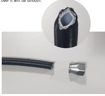
**3** After installing the nut onto the hose, flare out the stainless braid to make it easier to install the feral onto the PTFE Lining
