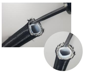
4 Once the braid has been pulled back, slide the feral onto the PTFE liner and press down until it is againce the lip shown below
