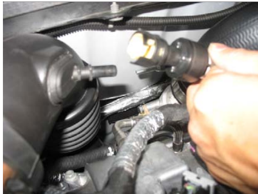
c) Disconnect the PCV line from the intake tube by pressing the clip and pushing back.
