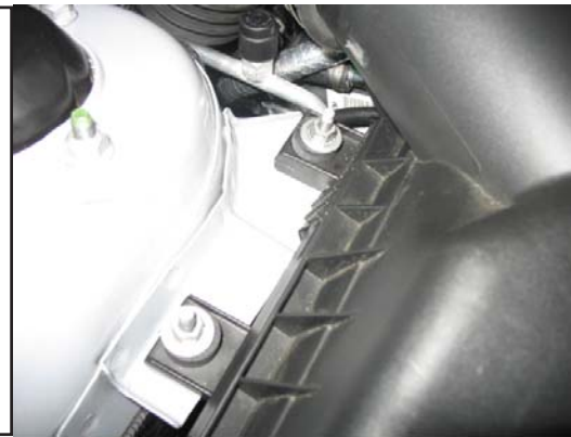
b) Remove the two 10mm nuts on the air box panel.
