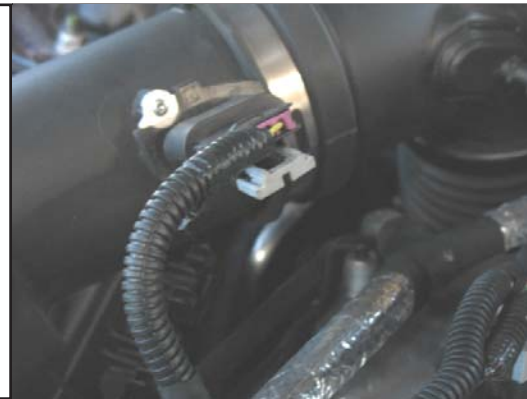
d) Remove the locking clip on the MAF sensor harness by pressing the clip with a small flathead screwdriver.
