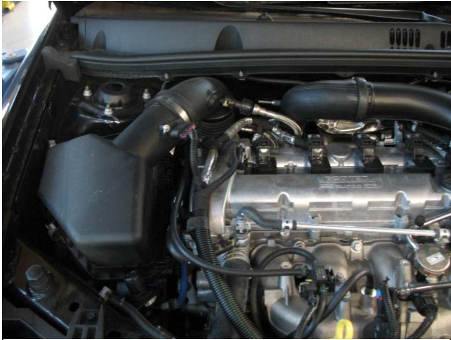
Stock Intake Installed
