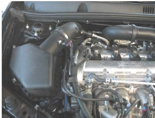
a) Stock intake installed
