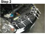
Remove (6) push pins located on top of the grill.
