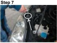
Remove (1) 10mm bolt located on top of the headlight.
