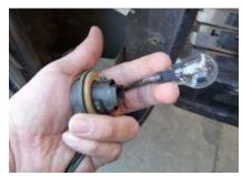
Step 4: Take off the bulb for the turn and brake light off the wire harness.
