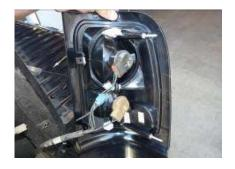
Step 6: Twist the light bulb wire harness into the new Anzo light.
