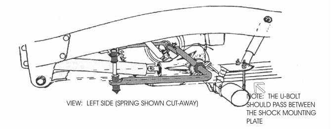
NOTE: ON PASSENGER SIDE OF FRAME, THE FRAME BRACKET MUST BE CENTERED OVER THE RIVET THAT ATTACHES THE SHOCK BRACKET TO THE FRAME.
