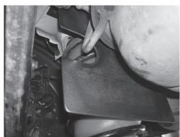
Make sure the slot in the heat shield is around the muffler mounting bracket.
