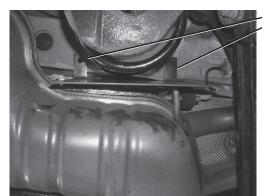
The heat shield attaches to the frame with self-tapping screws (D).
