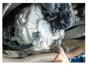
1. Remove the 4 flange nuts on the back of the factory cross member, but leave the bolts in place. Install 2 flat washers onto each bolt to act as spacers.
