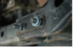
2. Install the ½" bolts with a flat washer into the 2 center holes in the cross member pointing rearward, then install 1 machined spacer onto the bolt on the other side of the cross member.
