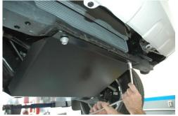
4. Now mount the Transmission Skid Plate to the rear of the IFS Skid and to the crossmember as pictured below using the supplied hardware:
