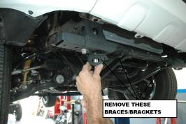
3. Install the All-Pro IFS Skid Plate in place of the factory skid plate using the factory hardware as shown below:
