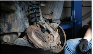
**3.** Remove all brake line mounts, wheel speed sensors, and related wiring from the knuckle (if equipped).
