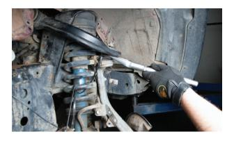
**9.** Remove the four 14mm bolts that attach the lower ball joint cradle to the knuckle.
