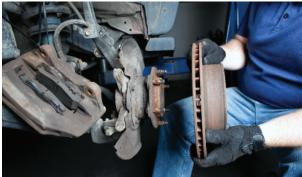
**5.** If the vehicle is equipped with 4WD, remove the dust cap exposing the axle nut. Remove the cotter pin and remove the axle nut using a 1 3/8" (or 35mm) socket.
