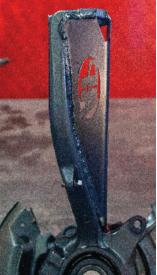
15. Position the provided gusset on the knuckle and mark the areas where the gusset contacts the knuckle. Remove any paint, grease, or other contaminants around the marked areas and prep the knuckle for welding. Minor sanding of the gusset may be required to achieve the best fit on the knuckle. Be sure to place the upper part of the gusset where it will not contact the ball joint or uniball puck when they are installed in the knuckle.
