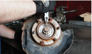
**6.** Loosen but do not remove the four 12mm bolts that hold the brake disc dust cover on the knuckle.
