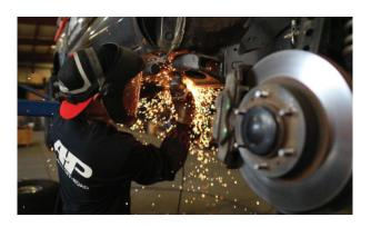
**9.** Grind off any remnants of the body mount be careful not cut grind into the frame too much.
