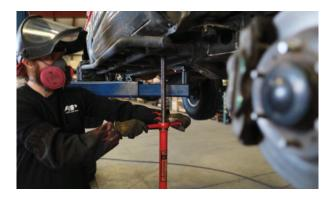
**8.** The body mount can be cut off using a plasma cutter, cutting torch, sawzall, or angle grinder. If using a sawzall or angle grinder the body mount bracket may need to be cut off in sections.
