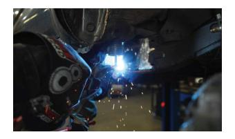
**15.** The inside and outside of the front and rear of the bracket along with the inside of the top will need to get welded.
