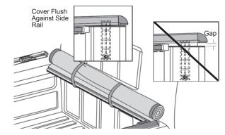
of each Side Rail, with the inside edge of the front bulkhead. Front of Bed Edge of Side Rail Tailgate must align with Inside Edge of Bed Inside Edge of Bed
