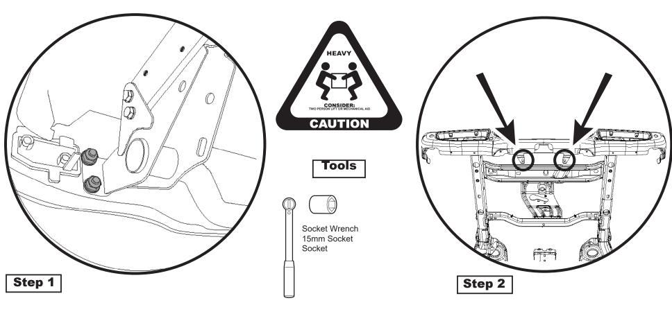
Use a socket wrench with a 17mm socket to remove the two (2) bolting into the rear of the factory bumper. Leave the bracket on the frame. Perform this on both L and R sides of the vehicle.
