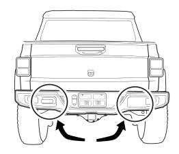
(If Equipped) The Bumper may be bolted to the bottom of the Tow-Bar with either a T50 ButtonCap bolt or a 16mm HexHead bolt.
