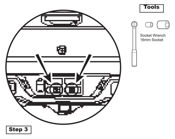
Remove the 16mm bolts behind the License Plate holder on the OEM bumper. Repeat on both bolts.
