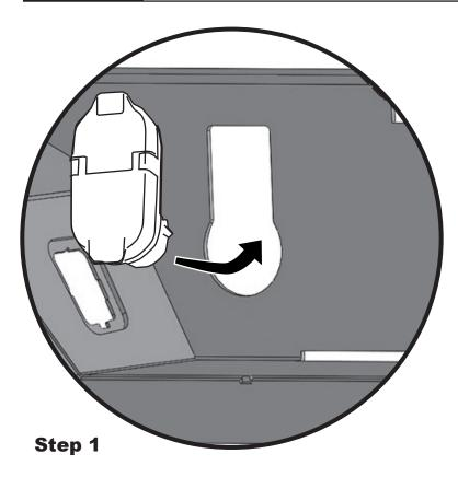
From the exterior side of the bumper: Re-install the Trailer Connector into the bumper Step as shown. Make sure that the Spring-Locks on the connector properly secure the connector body into the bumper.
