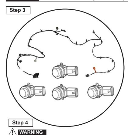
Note the Orientation of all the sensors, You will need to place them into the new bumper in the same manor. Remove all Parking and Driver assistance sensors and harnesses per dealership or vehicle manufacture service manuals. Take care with these components.
