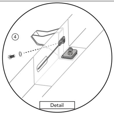
Tighten the 2 nuts that hold the Rear Bracket to the vehicle then tighten the three 12mm bolts that hold the Front Mounting Bracket to the vehicle.
