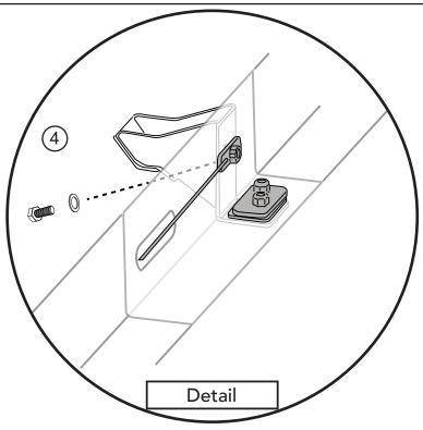
Tighten the 4 nuts that hold the Center and Rear Brackets to the vehicle then tighten the 3 12mm bolts that hold the front mounting Bracket to the Vehicle.
