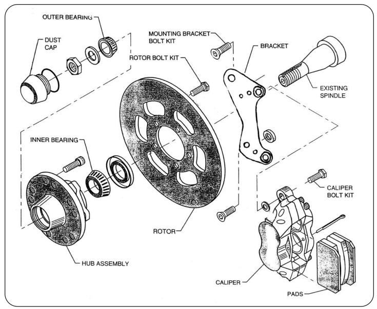
The Illustration is of a race kit. The street kit is the same except the rotor uses an adapter to bolt to the hub.
