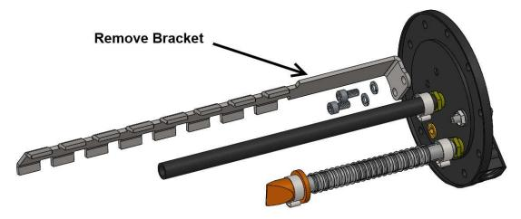
5. Remove the original fuel supply line from the standard Phantom fuel pump hanger assembly. To remove the original pinch clamp from the line, grasp the pinched portion of the clamp with a pair of pliers and twist to loosen.
