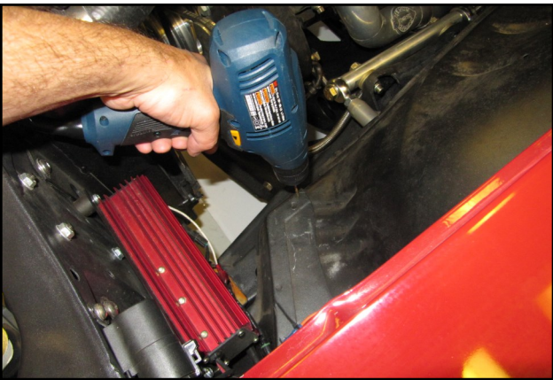
10. Drill 1/8" pilot holes into the inner fender.
