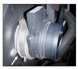
**8.** Slide the factory **MAF** sensor onto the air filter adapter and tighten the hose clamp. (*Note: factory clamp / rubber bushing must be in place on the inlet to the MAF sensor.)*
