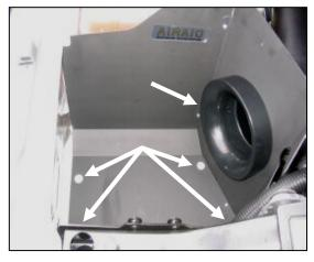
7. Install the air filter adapter (#4) using three  $\frac{1}{4}$ -20x  $\frac{1}{2}$ " button head bolts (#12), and 1/4" flat washers (#13). Position the Airaid Cool Air Dam in place of the factory airbox & secure it with four M6-1x25 hex bolts (#14) and 1/4" flat washers (#13).
