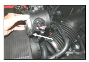
2. Remove the Mass Air Flow sensor from between the factory intake tube and the factory air box. Use caution to retain the rubber coupler on the Mass Air Flow sensor.
