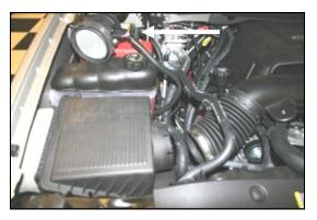
**3.** Without disconnecting the wiring harness, set the Mass Air Flow sensor out of the work area. Next rock the factory air box back and forth, lift it up, and remove it from the hold down grommets. There are no bolts holding it down.
