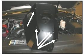
6. Assemble the two Cool Air Dam panels (#2) and (#2) and (#2)
