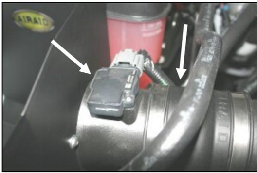
10. Reinstall the MAF sensor onto the filter adapter using two 8-32 x 5/8" Allen Bolts (#13).
