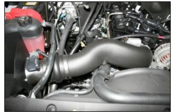
12. Install the Airaid Intake Tube into the hump hose first, and then onto the throttle body. Adjust it for fit, and then tighten all three hose clamps. Reinstall the plastic retainer on the radiator hose into the bottom of the Airaid Intake Tube. Refer to step #3.
