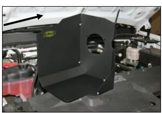
**5.** Assemble the two Cold Air Dam (CAD) panels (#2 & #3) using five 6-32 Phillips screws (#6) five flat washers (#7), and five keps nuts (#8) as shown. Make sure that panel #2 is located inside of panel #3.
