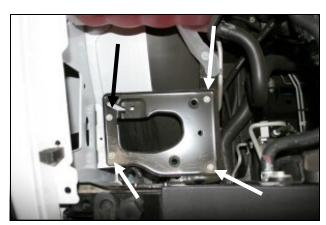
**4.** Using a 10mm socket, remove the four bolts that secure the factory airbox mounting plate. Now remove the mounting plate from the vehicle.
