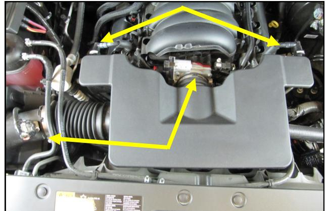
5. Reinstall the intake system and tighten the two hose clamps. Reconnect the valve cover breather lines.
