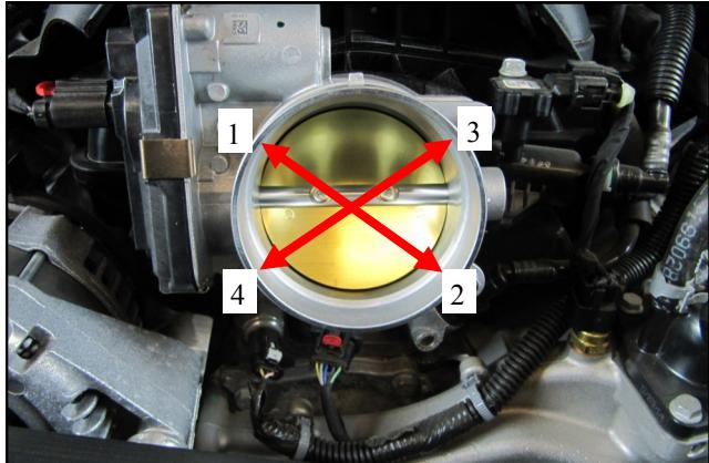
4. Insert the provided bolts with washers through the throttlebody, gasket, and Poweraid Spacer and tighten them in an “X” Pattern.
