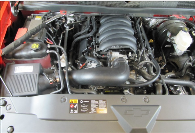
13. Double check your work. Make sure all Clamps are tight and reconnect the negative battery cable.
